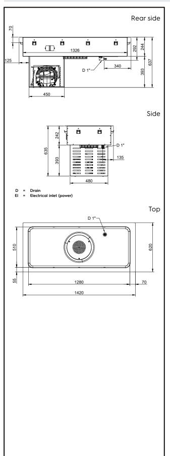
Drop-In Drop-in refrigerated well, static with fan (4 GN container capacity)
