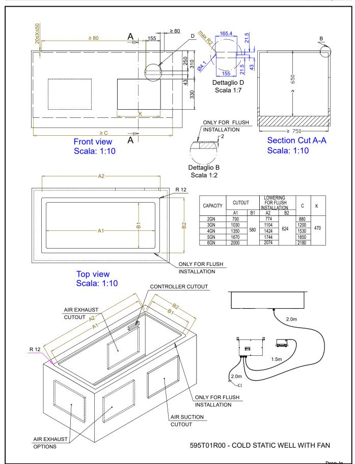
Drop-in refrigerated well, static with fan (4 GN container capacity)
